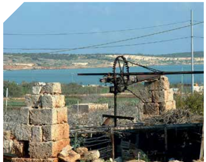
Water stored above the blue clay layer used to be pumped up by means of the water pump (the remains of the machinery are visible in the picture above) or with a wind-pump (See picture below). Water was used to irrigate the fields especially during the dry summer months.
