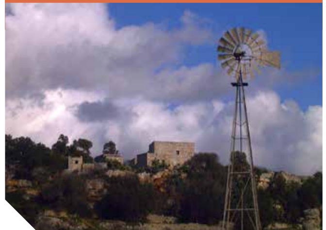
Water stored above the blue clay layer used to be pumped up by means of the water pump (the remains of the machinery are visible in the picture above) or with a wind-pump (See picture below). Water was used to irrigate the fields especially during the dry summer months.
