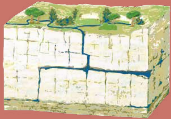
Water percolates through the cracks and joints in the rocks.
